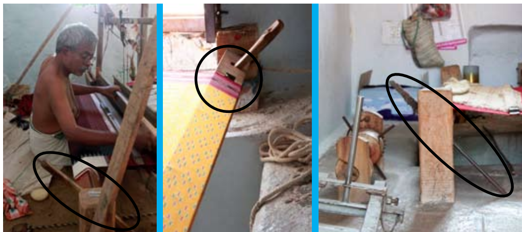
Stick used as an anti-rolling device, length depends upon height of loom
