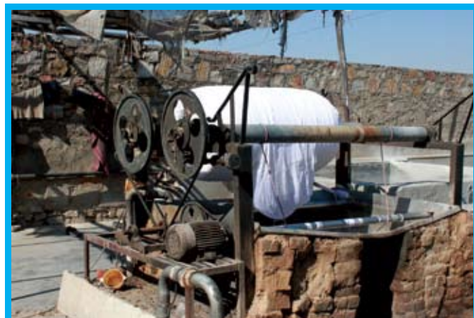
Wax removal machine in Ikat
